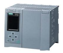
SIMATIC S7-1500F, CPU 1518F-4 PN/DP, central processing unit with 9 MB work memory for program and 60 MB for data, 1st interface: PROFINET IRT with 2-port switch, 2nd interface: PROFINET RT, 3rd interface: PROFINET basic services, 4th interface: PROFIBUS, 1 ns bitperformance, SIMATIC Memory Card required
