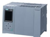
SIMATIC S7-1500H, CPU 1517H-3 PN, central processing unit with 2 MB work memory for program and 8 MB for data, 1st interface: PROFINET RT with 2-port switch, 2nd interface: PROFINET, 3rd/4th interface: H-SYNC, SIMATIC Memory Card required
