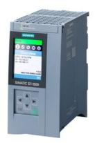
SIMATIC S7-1500, CPU 1515-2 PN, central processing unit with 500 KB work memory for program and 3 MB for data, 1st interface: PROFINET IRT with 2-port switch, 2nd interface: PROFINET RT, 30 ns bit performance, SIMATIC Memory Card required
