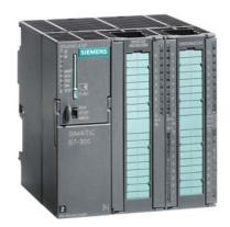
SIMATIC S7-300, CPU 314C-2 DP Compact CPU with MPI, 24 DI/16 DO, 4 Al, 2 AO, 1 Pt100, 4 high-speed counters (60 kHz), integrated DP interface, Integr. power supply 24 V DC, work memory 192 KB, Front connector (2x 40-pole) and Micro Memory Card required
