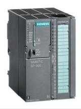
SIMATIC S7-300, CPU 312C Compact CPU with MPI, 10 DI/6 DQ, 2 high-speed counters (10 kHz) Integr. power supply 24 V DC, work memory 64 KB, Front connector (1x 40-pole) and Micro Memory Card required
