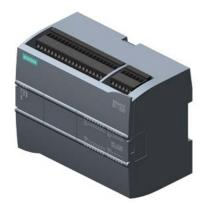
SIMATIC S7-1200, CPU 1215C, compact CPU, DC/DC/relay, 2 PROFINET ports, onboard I/O: 14 DI 24 V DC; 10 DO relay 2 A, 2 AI 0-10 V DC, 2 AO 0-20 mA DC, Power supply: DC 20.4-28.8 V DC, Program/data memory
