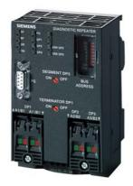
SIPLUS DP diagnostic repeaters based on 6ES7972-0AB01-0XA0 with conformal coating, 0...+60 °C,
