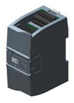
SIPLUS S7-1200 SM 1221 16DI based on 6ES7221-1BH32-0XB0 with conformal coating, -40...+70 °C, start up -25 °C, digital input 16 DI, 24 V DC, sink/source
