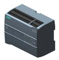
SIPLUS S7-1200 CPU 1215C DC/DC/DC based on 6ES7215-1AG40-0XB0 with conformal coating, -20...+60 °C, compact CPU, DC/DC/DC, 2 PROFINET ports, onboard I/O: 14 DI 24 V DC 10 DQ 24 V DC 0.5 A 2 AI 0-10 V DC, 2 AQ 0-20 mA DC, power supply: DC 20.4-28.8 V DC, program/data memory 125 KB
