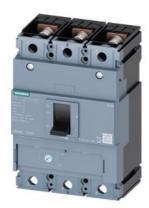
circuit breaker 3VM1 IEC frame 250 breaking capacity class N Icu=25kA @ 415V 3-pole, line protection TM220, ATFM, In=200A overload protection Ir=140A...200A short-circuit protection Ii=10 x In nut keeper kit
