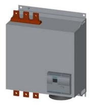
SIRIUS soft starter Values at 400 V, 40  $^{\circ}\text{C}$  standard: 693 A, 400 kW Inside-delta: 1200 A, 710 kW 200-460 V AC, 230 V AC Screw terminals !!! Phased-out product !!! Successor is SIRIUS 3RW5, Preferred successor type is >>3RW5553-6HA14<<
