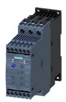
SIRIUS soft starter S0 25 A, 11 kW/400 V, 40  $^{\circ}\text{C}$  200-480 V AC, 24 V AC/DC Screw terminals Thermistor motor protection
