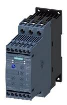
SIRIUS soft starter S0 12.5 A, 5.5 kW/400 V, 40 °C 200-480 V AC, 24 V AC/DC Screw terminals Thermistor motor protection
