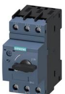
Circuit breaker size S0 for motor protection, CLASS 10 A-release 16...22 A N-release 286 A screw terminal Standard switching capacity
