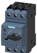
Circuit breaker size S0 for motor protection, CLASS 10 A-release 7...10 A N release 130 A screw terminal Standard switching capacity
