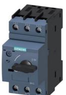
Circuit breaker size S0 for motor protection, CLASS 10 A-release 1.8...2.5 A N-release 33 A screw terminal Standard switching capacity
