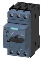
Circuit breaker size S0 for motor protection, CLASS 10 A-release 1.4...2 A N-release 26 A screw terminal Standard switching capacity
