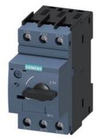
Circuit breaker size S0 for motor protection, CLASS 10 A-release 0.9...1.25 A N-release 16 A screw terminal Standard switching capacity
