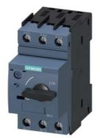
Circuit breaker size S00 for motor protection, CLASS 10 A-release 0.22...0.32 A N-release 4.2 A screw terminal Standard switching capacity
