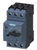
Circuit breaker size S00 for motor protection, CLASS 10 A-release 0.11...0.16 A N-release 2.1 A screw terminal Standard switching capacity
