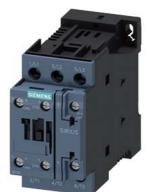
power contactor, AC-3e/AC-3, 38 A, 18.5 kW / 400 V, 3-pole, 24 V DC, auxiliary contacts: 1 NO + 1 NC, screw terminal
