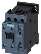
power contactor, AC-3e/AC-3, 25 A, 11 kW / 400 V, 3-pole, 230 V AC, 50 Hz, auxiliary contacts: 1 NO + 1 NC, screw terminal
