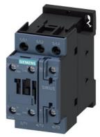
power contactor, AC-3e/AC-3, 17 A, 7.5 kW / 400 V, 3-pole, 230 V AC, 50 Hz, auxiliary contacts: 1 NO + 1 NC, screw terminal
