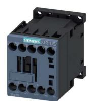
power contactor, AC-3e/AC-3, 16 A, 7.5 kW / 400 V, 3-pole, 24 V DC, auxiliary contacts: 1 NO, screw terminal
