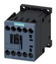
power contactor, AC-3e/AC-3, 12 A, 5.5 kW / 400 V, 3-pole, 24 V DC, auxiliary contacts: 1 NO, screw terminal
