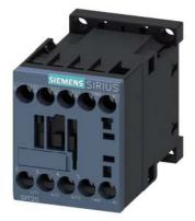
power contactor, AC-3e/AC-3, 12 A, 5.5 kW / 400 V, 3-pole, 230 V AC, 50/60 Hz, auxiliary contacts: 1 NO, screw terminal
