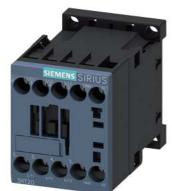
power contactor, AC-3e/AC-3, 9 A, 4 kW / 400 V, 3-pole, 230 V AC, 50/60 Hz, auxiliary contacts: 1 NO, screw terminal
