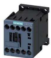
power contactor, AC-3e/AC-3, 7 A, 3 kW / 400 V, 3-pole, 24 V DC, auxiliary contacts: 1 NO, screw terminal
