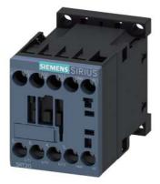
power contactor, AC-3e/AC-3, 7 A, 3 kW / 400 V, 3-pole, 230 V AC, 50/60 Hz, auxiliary contacts: 1 NO, screw terminal
