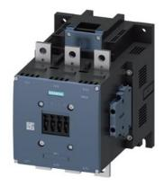
power contactor, AC-3e/AC-3 500 A, 250 kW / 400 V AC (50-60 Hz) / DC Uc: 220-240 V 3-pole, auxiliary contacts 2 NO + 2 NC drive: conventional main circuit: busbar control and auxiliary circuit: screw terminal
