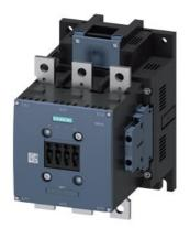
power contactor, AC-3e/AC-3 265 A, 132 kW / 400 V AC (50-60 Hz) / DC Uc: 220-240 V 3-pole, auxiliary contacts 2 NO + 2 NC drive: conventional main circuit: busbar control and auxiliary circuit: screw terminal
