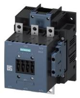
power contactor, AC-3e/AC-3 185 A, 90 kW / 400 V AC (50-60 Hz) / DC Uc: 220-240 V 3-pole, auxiliary contacts 2 NO + 2 NC drive: conventional main circuit: busbar control and auxiliary circuit: screw terminal
