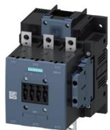
power contactor, AC-3e/AC-3 150 A, 75 kW / 400 V AC (50-60 Hz) / DC Uc: 220-240 V 3-pole, auxiliary contacts 2 NO + 2 NC drive: conventional main circuit: busbar control and auxiliary circuit: screw terminal
