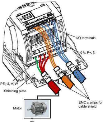
The following diagram shows an example of EMC-compliant installation of the converter frame size B/C.
