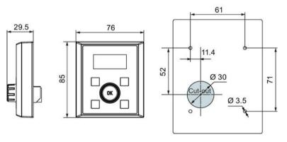
Unit: mm Fixings: 4 x M3 screws (length: 8 mm to 12 mm) Tightening torque: 0.8 Nm ± 10%
