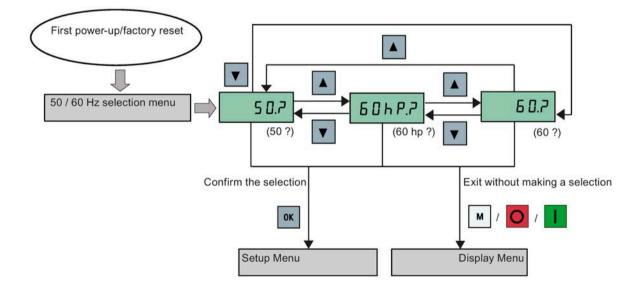
5.4 Starting the motor for test run
