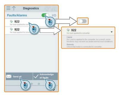
You can use the filter button to display all faults and alarms or the active ones only.
