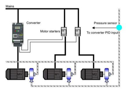
The diagram below shows a typical pumping system.
