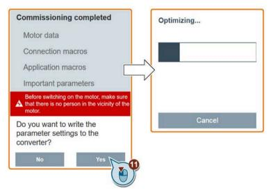
9. Confirm completion of the quick commissioning when the following window appears. If the Web page indicates that the optimization fails, you can select to try optimization again.
