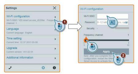
Note that the new Wi-Fi configuration takes effect only after the SINAMICS V20 Smart Access restarts.
