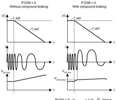
P1254 = 0:  $V_{DC-Comp} = 1.13 \cdot \sqrt{2} \cdot P0210$ P1254  $\neq$  0:  $V_{DC-Comp} = 0.98 \cdot r1242$
