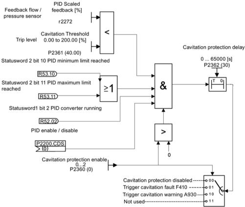
**Cavitation Protection Logic Diagram**
