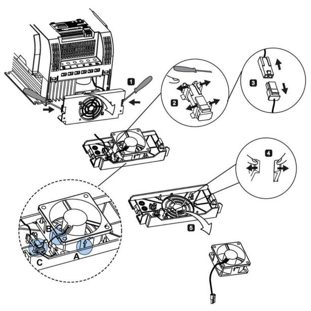
Replacing the fans from FSE
