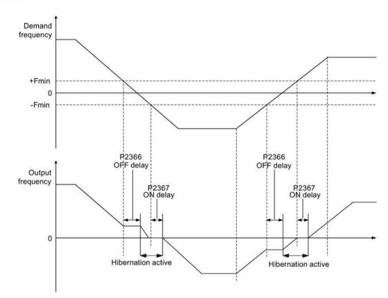
• PID hibernation: When the converter under PID control drops below the PID hibernation setpoint (P2390), the PID hibernation timer (P2391) is started. When the timer expires, the converter is ramped down to stop and enters the hibernation mode. The converter restarts when it reaches the PID hibernation restart point (P2392).
